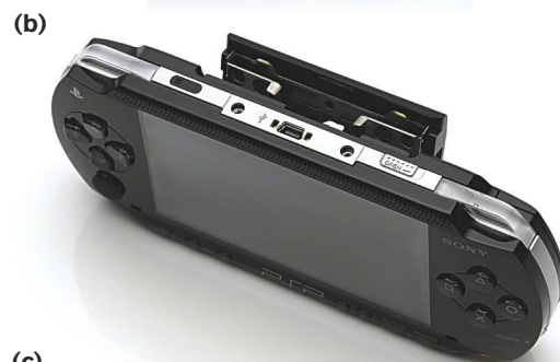
(c) Figure 3 The PSP's beefy, multicore CPU and graphics subsystem, along with other enhanced hardware capabilities, deliver highly detailed games (a). The system can also function as a USB mass-storage device and as an audio, still-image, and video player (b). The video-player function employs content streamed over or downloaded from the Internet from a Memory Stick or on a Sony-proprietary UMD optical disc (c).
