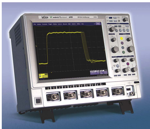
WaveRunner Xi scopes provide the performance of larger and costlier instruments in a 6-in.-deep package with an 800X600-pixel, 10.4-in. screen.
